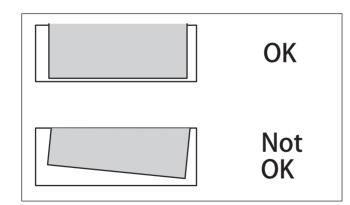
After loading, check the following points. ➤ The media is loaded straight.
