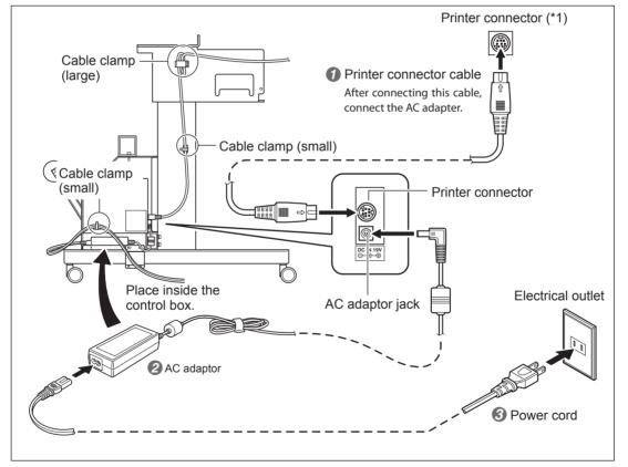
(\*1) The position of the printer connector differs depending on the model. On the VG series, the connector is located on the front of the printer, below the heater. On the VS series, the connector is located on the back of the printer, close to the power supply.
