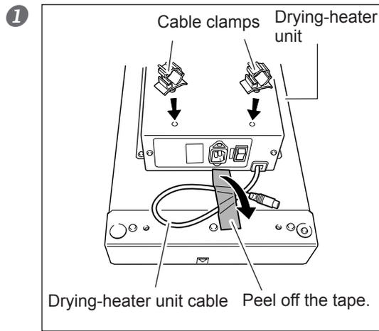
Peel off the tape holding the drying-heater unit cable in place and attach cable clamps at the locations shown in the figure.
