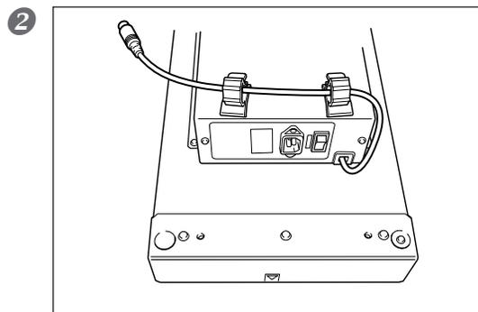
Pass the drying-heater unit cable through the cable clamps.
