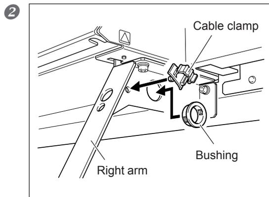
Attach the bushing and cable clamp to the right arm.
