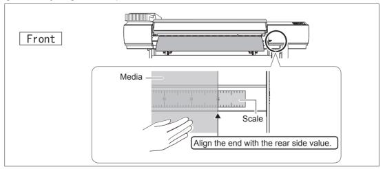
3. If the difference between the rear and front scale values indicating the position of the media is 1 mm or more, redo to adjust the position of media.
