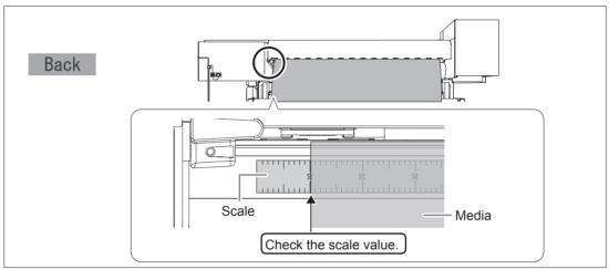
2. Adjust the position of the media on front of the printer so that its position passes through the scale marks with the same value\* on rear side of the printer.
