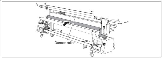
2 Lower the height of media supports to the bottom by rotating the lever. Be sure the media supports are set in the inner side of the both media holders first, and rotate the lever of the media supports in the direction of the arrow shown in the figure.
