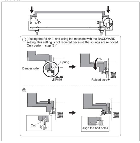
3 Attach the end of the dancer roller on the frame side with the same procedure 1.2.
