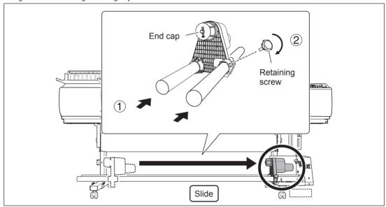
**5** ① Slide the media holder L onto the shafts.
